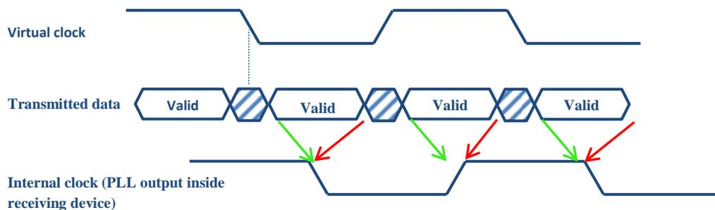
Note, the arrows above show which data transition point is used for setup and hold and the corresponding latch clock edges.
