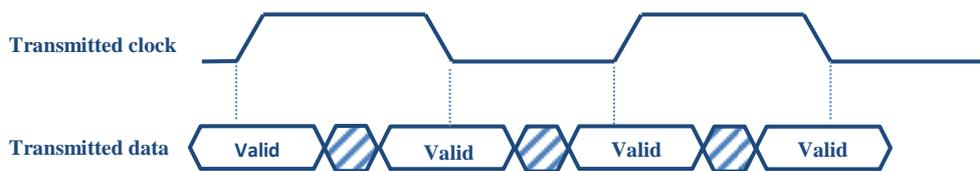
The performance of such an interface could be specified as skew such as  $\pm 0.25\text{ns}$  with a defined clock offset(ideally 90 degrees).
