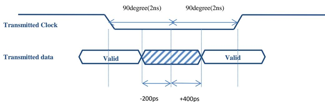
(If the clock to data relationship is specified using setup & hold parameters then the skew can be calculated from these figures.)
