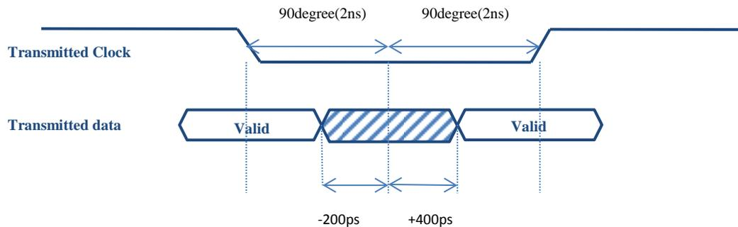
(If the clock to data relationship is specified using setup & hold parameters then the skew can be calculated from these figures.)
